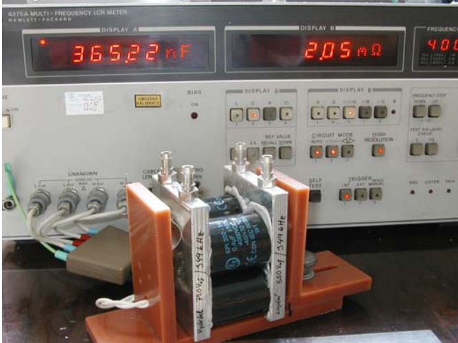
Measurement of the capacitors
