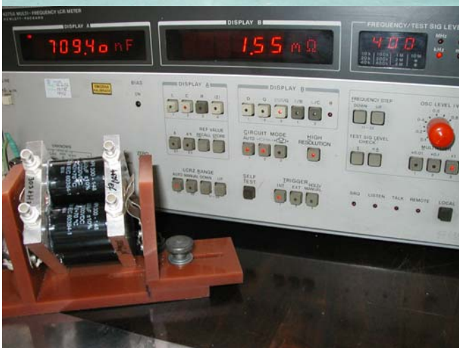
Measurement of the capacitors at 400kHz
